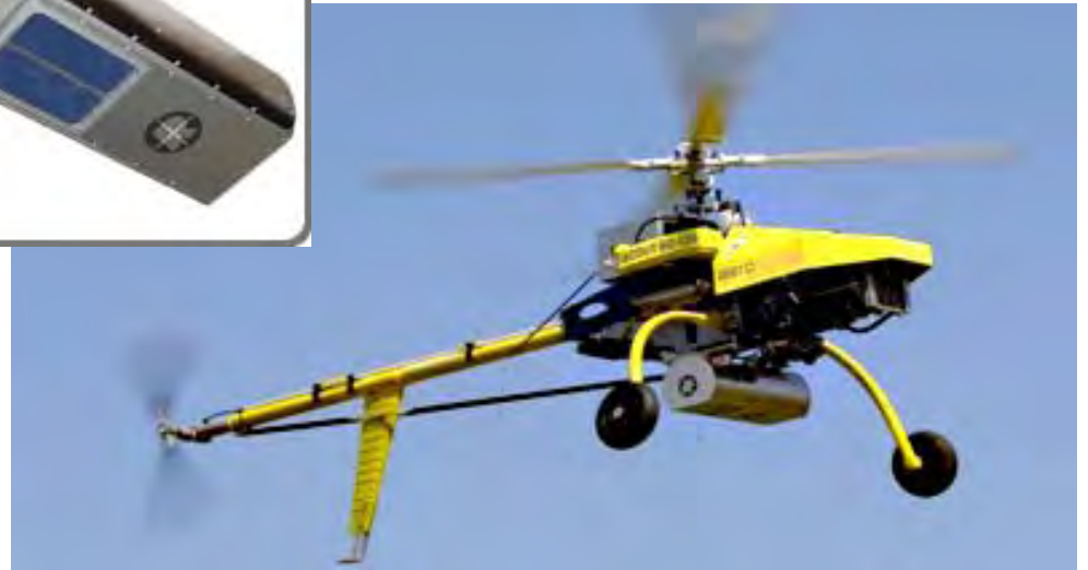
UAV with lidar sensor
