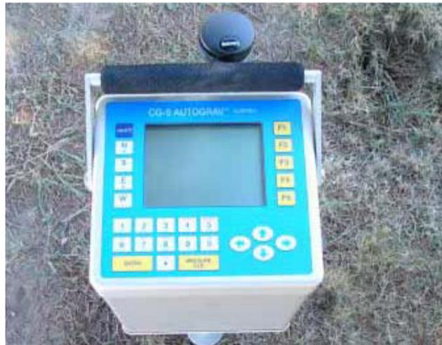
**Figura 2.4. 2.** Gravímetro Scintrex Autograv CG-5 (Scintrex limited,2012).
